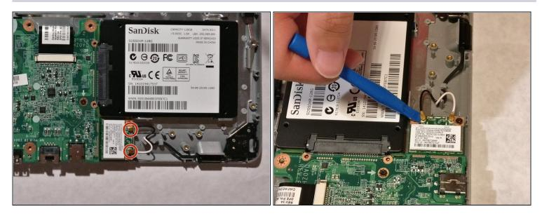
• Remove the two antenna cables from the wireless card. These should snap lightly out of place when lifted upwards.
