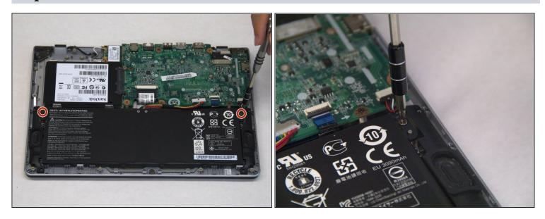
• Unscrew the two 6.2 mm Phillips #1 head screws on either side of the battery as indicated.
