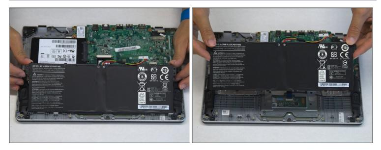
• Lift the battery up and off the rest of the laptop.
