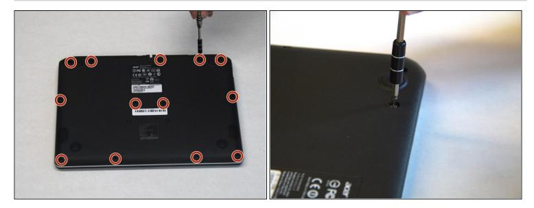
• Remove the 13 indicated screws (6.2 mm) using a Phillips #1 screwdriver.
