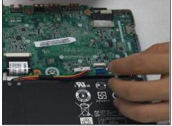
• Dislodge the battery's connector to the motherboard by using the plastic opening tool as a lever on the two small plastic tabs that stick out on either side of the connector.
