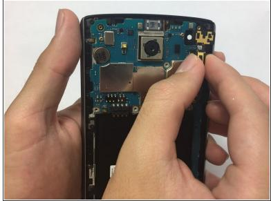
Using the flat end of a plastic spudger or a plastic opening tool, wedge it under the front cameras' motherboard connection and disconnect it. After replacing the dual front cameras, follow these instructions in reverse order to reassemble the LG V10.
