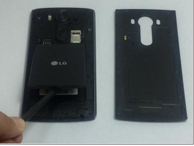
There's an impression next to the battery for the user to use their finger to pry the battery out; pry
