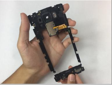
Carefully but firmly pull on the loudspeaker component to release it from the plastic bits holding it in place. After replacing the loudspeaker, follow these instructions in reverse order to reassemble the LG V10.
