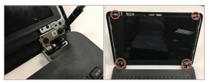
• Remove the two 5/16 screws in the top corners and the four in the bottom corners.
