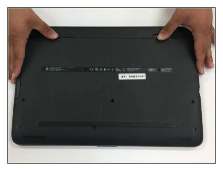
Slide the two battery lock latches on the back of the device to the "unlock" position.
