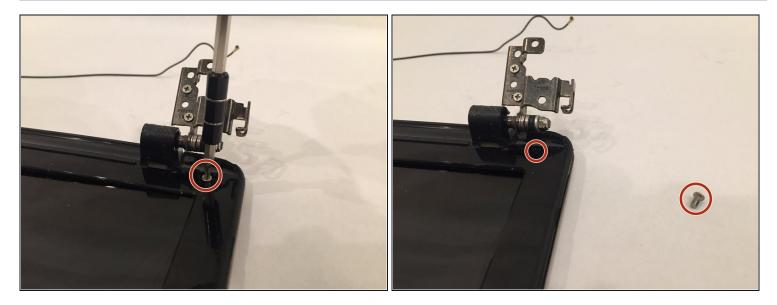
• Unscrew the two 1.5mm screws at the bottom of monitor using a Philips #0 screwdriver.
