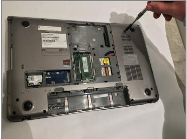
• Remove the fourteen (14) screws using a Philips #0 screwdriver for the 1.5mm screws on the underside of casing.
