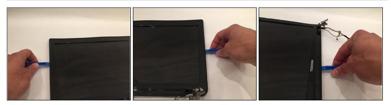
• Using a prying tool, carefully pry along the edges of the screen cover
