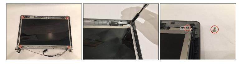
• Using the Philips #0 screwdriver, remove the four 1.5mm screws at the corners of the screen.
