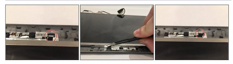
• At the top of the screen, using the tweezers, remove the ZIF ribbon connector by gently pushing it up.
