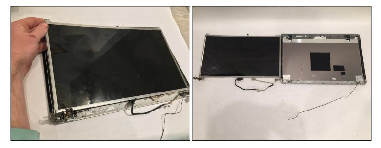
• Remove the screen from the device.
