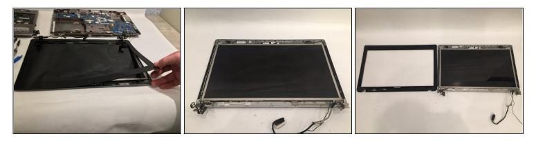
• With all the edges of the screen cover pried up, carefully remove the screen cover.
