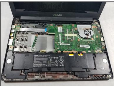
Lift the keyboard assembly away from the remainder of the laptop.
