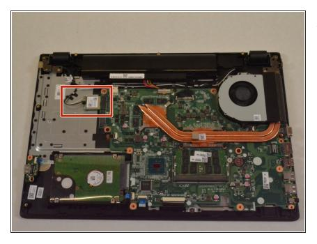
Locate the wireless card on the top left quadrant. It should have two antenna cables connected to it, one white and one black.
