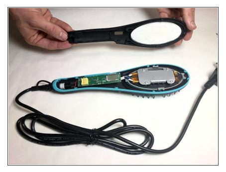
Now that the screws are taken out, remove the backside of the comb.
