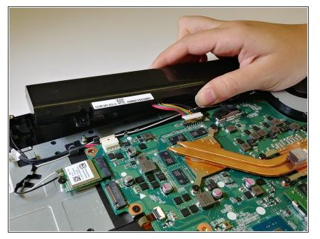
• Lift the battery directly up to remove it from the laptop. It is not screwed on.
