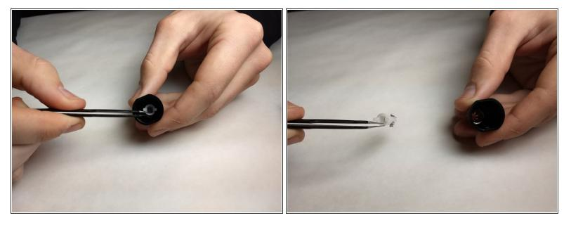
Using the tweezers, pull the blade assembly out of the trimmer tip.
