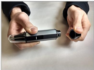
Twist the battery cap found on the bottom of the device counterclockwise.
