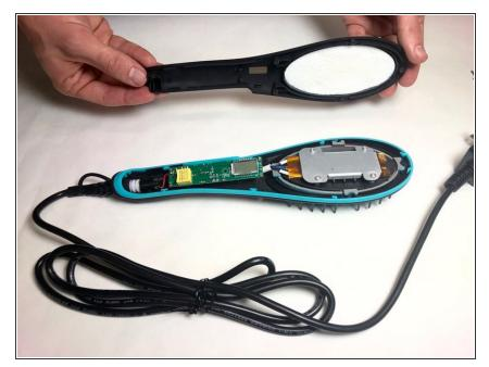
• Now that the screws are taken out, remove the backside of the comb.
