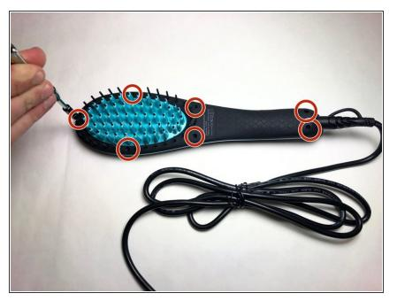
Remove the seven 5mm Phillips #1 screws on the comb-side of the brush.
