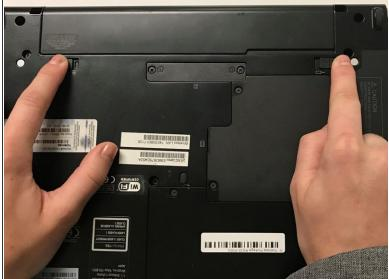
Unlock the clips by pulling towards the open lock.
