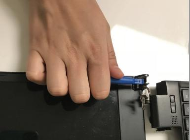
Remove the chrome hinges using the blue prying tool. The hinges should pop right off without must effort.
