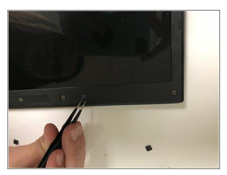
Using tweezers, remove the plastic caps from the top edge of the laptop screen, located near the front-facing camera. All but the cap closest to the camera should be removed.
