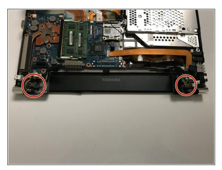
Remove the screw from the metal hinges in the top corners of the laptop as shown in the picture.
