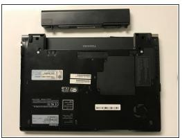
Hold the unlock clip while pulling the battery away from the laptop.
