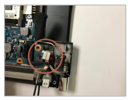
Disconnect the white plug with red and black wires located on the rightmost upper corner with the chrome hinges pointed farthest away from you.
