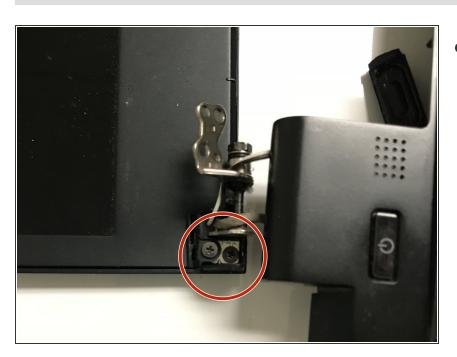
Remove the screws located underneath the hinges.
