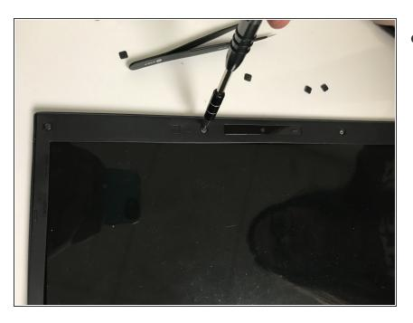
Remove the screws located underneath the plastic caps.
