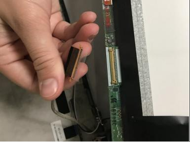
• Disconnect the grey mesh wire from underneath the unattached laptop screen.
