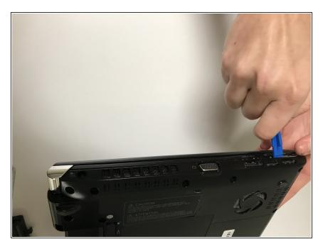
Use the plastic tool to help pry the back off of the laptop
