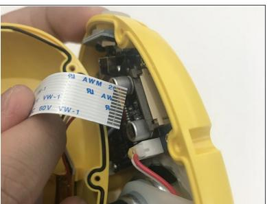
Using the plastic opening tool pull up the black tab up until it stops.
