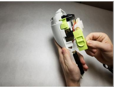
Replace the new switch by sliding the replacement switch onto the top of the switch mechanism located on the motor.
