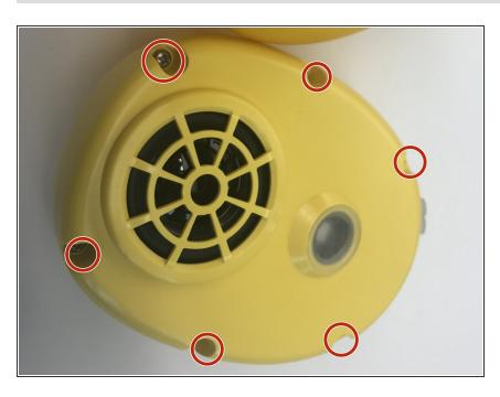
Using the J1 screwdriver bit, unscrew all six 9 mm screws that run along the border.
