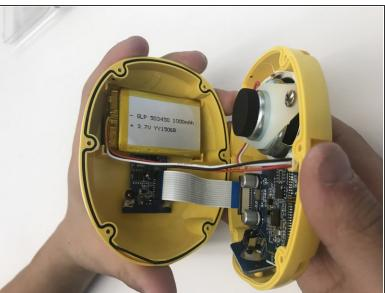
Use the plastic opening tool to open the inside of the duck.
