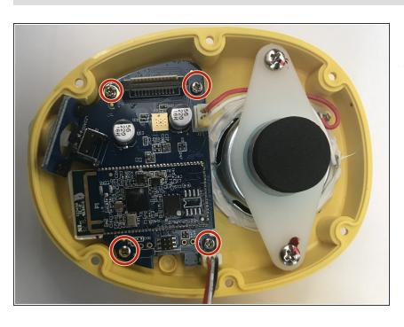
Use the J1 screwdriver bit to unscrew all four 9 mm screws attached to the motherboard.
