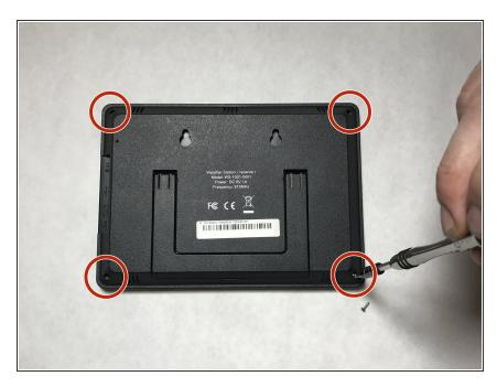
First, you will need to remove all four M2x1-7 screws (7mm length) located on the back of the device. This should be done using a Phillips #1 screw driver.
