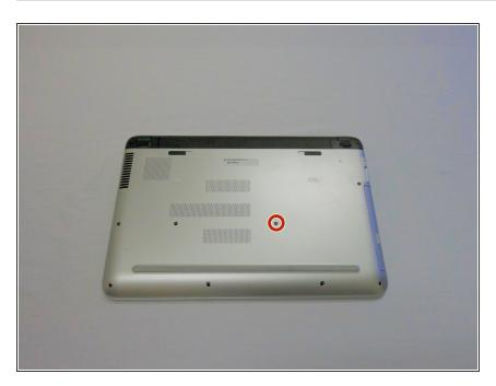
Remove the 8mm screw holding the optical drive in place with a Philips #1 screwdriver.
