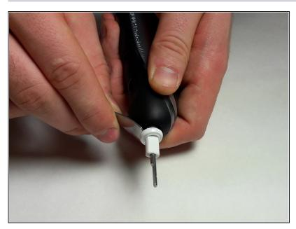
Remove the top cap by using a spudger to pry the plastic ring off of the toothbrush frame.
