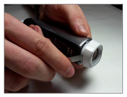
Remove the end cap from the bottom of the toothbrush by prying it off with a spudger.
