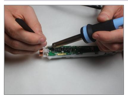
Melt the solder at the two pads on either side of the top of the motherboard. This will require a high heat soldering iron. Remove the wire from the solder pads using tweezers once the solder melts.
