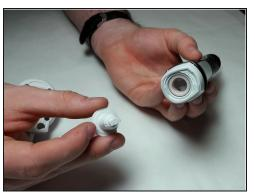
• Use the charging station to remove the a small plastic plug from the end of the toothbrush by inserting the charging station into the end insert and twisting counterclockwise by 90 degrees.
