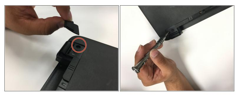
In the same spot you've just removed the bumpers from, you will find two 5/16 in. screws. Using the same Phillips-head screwdriver used in step 2, remove the screws
