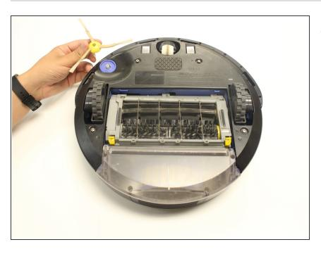
Gently pull the brush up and remove it from the device.
