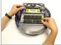
Press lightly on the yellow tabs and lift the cage cover containing the brush.
