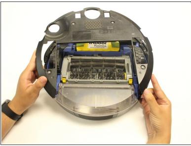
Remove the four 10mm screws with a Phillips #1 screwdriver. Gently lift off the external covering for the Roomba's underside.
