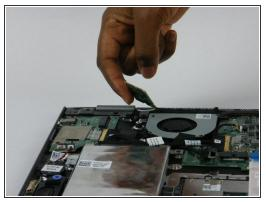
Unscrew the 2mm screw that holds the WLAN card. Then carefully remove the WLAN card from the motherboard.
