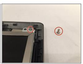
Using the Philips #0 screwdriver, remove the four 1.5mm screws at the corners of the screen.
