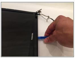
Using a prying tool, carefully pry along the edges of the screen cover
