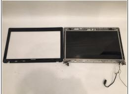
• With all the edges of the screen cover pried up, carefully remove the screen cover.
