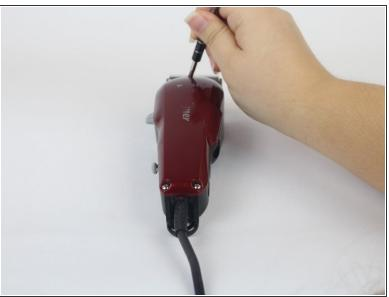
Unscrew the 12 mm Phillips head screws located at the top of the cover and at the bottom two corners, using a Phillips #1 Screwdriver.
