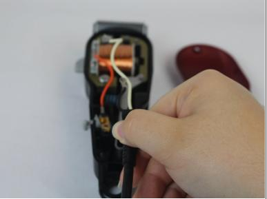
Remove the power cord from its mount at the bottom of the device.
