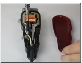
Unscrew the black 5.556 mm Phillip head screw on the power switch, closest to the power cord with a Phillips #0 Screwdriver.
