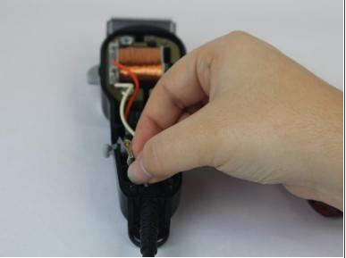
Gently remove the black wire connected to the black screw.
