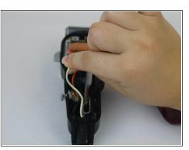
Remove the white wire connected to the power cord and the motor by grabbing the white wire firmly on both sides near the motor mounting and wiggling until release.
