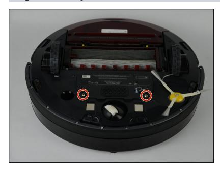
Flip over the device and remove the two 11.5 mm screws using the Phillips #1 screwdriver.
