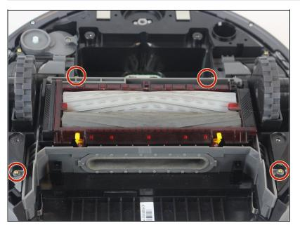
Remove the (4) 15.8mm Phillips #1 gold screws around the brush module.
