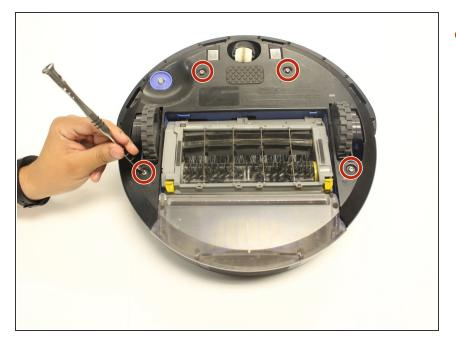
Unscrew the four 10mm screws on the underside of the Roomba using a Phillips #1 screwdriver.
