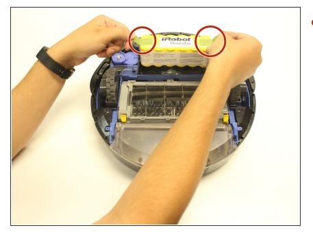
Grab the green tape attached to the end of the battery and remove the battery from the device.
