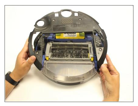
• Remove the bottom frame of the device.
