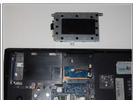
Remove the hard drive from the laptop by using a Spudger tool to pry it out.
