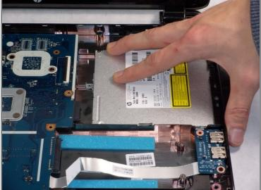
• Slide the CD drive out slowly by pulling it to the right. There are no screws attached, but there is a connection to the motherboard.
