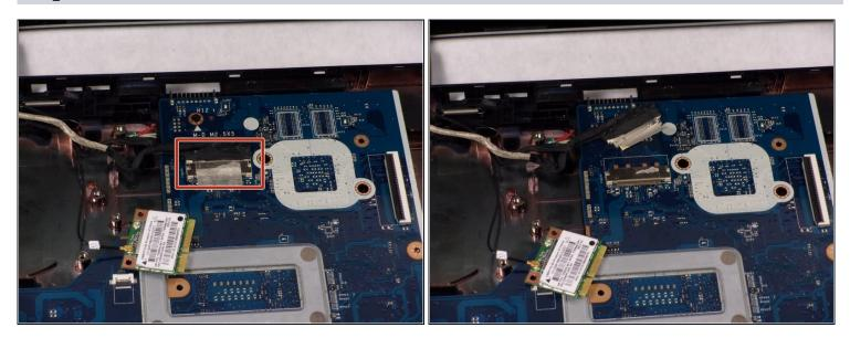
Lift up tape, and then remove the power cable from its connector.
