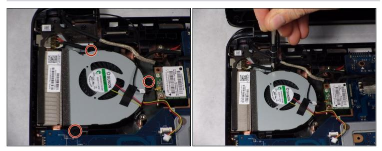
• Remove the three (3) 2.5mm by 3.5mm Phillips #0 screws from the fan.
