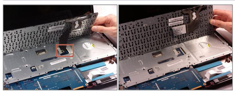
Disconnect the connection between the keyboard the the motherboard.
