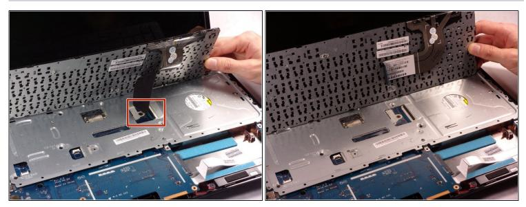
Disconnect the connection between the keyboard the the motherboard.
