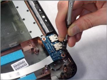
• Remove the one (1) 2.5mm by 3.5 mm Phillips #0 screw from the USB port plate.
