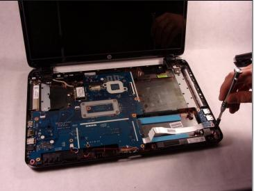
• Remove the four (4) 2.5 mm Phillips #0 screws.
