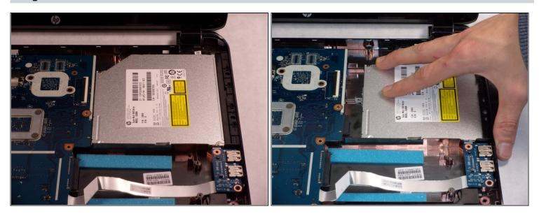
• Slide the CD drive out slowly by pulling it to the right. There are no screws attached, but there is a connection to the motherboard.
