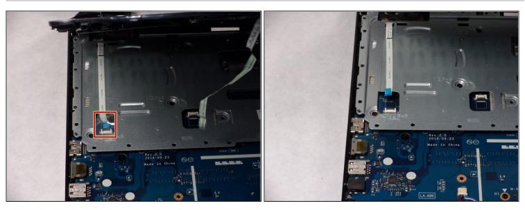
• Locate the connection between the power button and the connecting cable.
