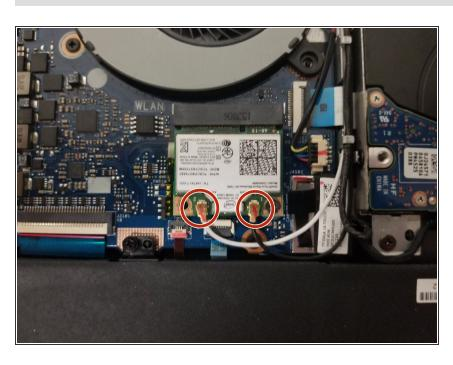
Disconnect the WiFi antennae by gently pulling up at each antenna's connector. Use a spudger to help lift each antenna free from the WiFi card if needed.
