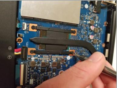
• Use a Phillips #0 screwdriver to remove the four 3 mm screws that secure the heat sink.
