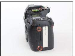
Using a Philips #00 screwdriver, remove the four 6.2mm from the left and right sides of the outer cover.
