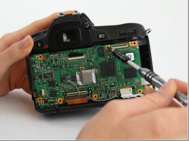
Use a Phillips #00 screwdriver to unscrew the 2.3 mm screw.
