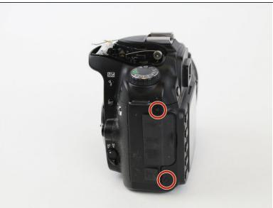
Using a Phillips #00 screwdriver, remove the four 6.2 mm screws from the left and right sides of the outer cover.
