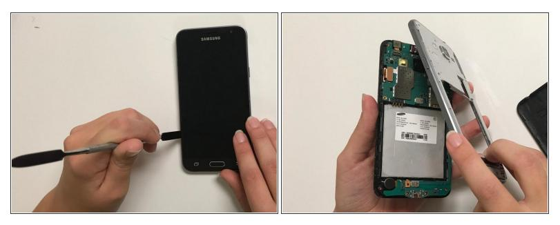
• Use the flat side of the metal spudger to remove the middle frame bezel.
