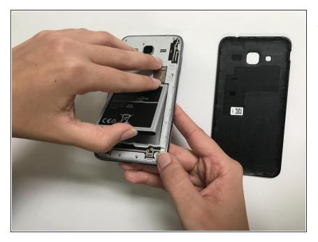
Remove the battery by gripping on and pulling up.
