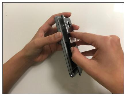
Separate the back casing from the phone by carefully using your fingers to pry it apart.
