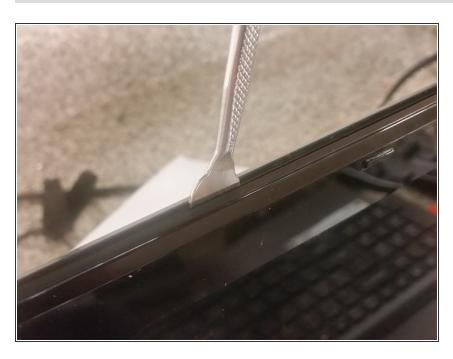
Use a spudger to remove the bezel.
