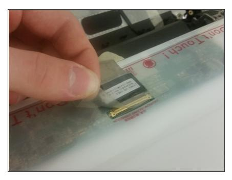
Separate all of the tape from the back of the LCD screen, and then pull straight back on the cable to remove it from the LCD.
