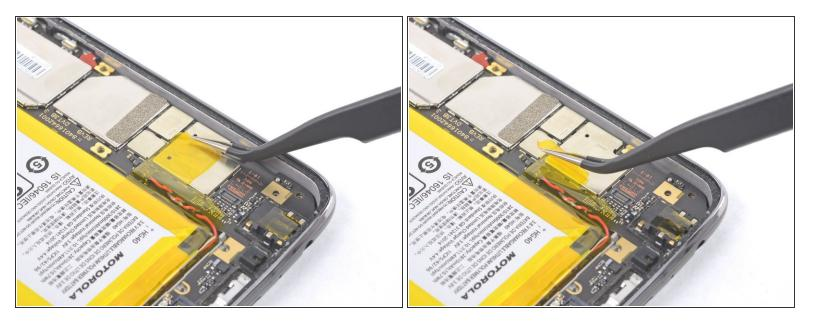
Remove the yellow tape covering the battery connector.
