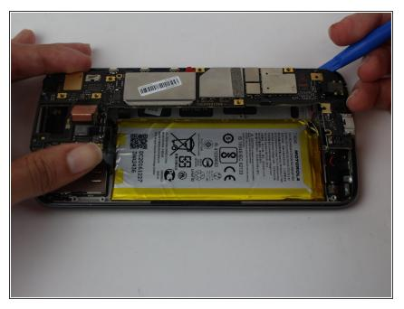
Using the plastic opening tool, pry open the two tabs that hold the motherboard to the phone frame.
