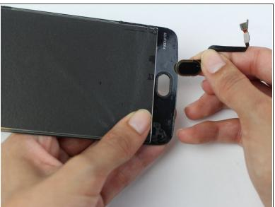
Remove the fingerprint sensor button from the screen by pushing it out with your fingers.
