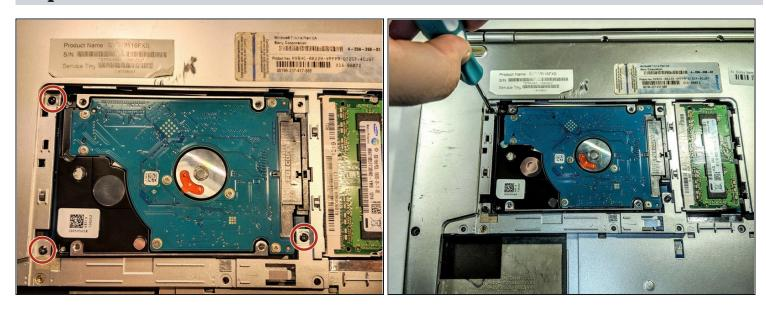
• Remove the three 5mm Phillips head screws that secure the Hard Drive bay to the back panel.
