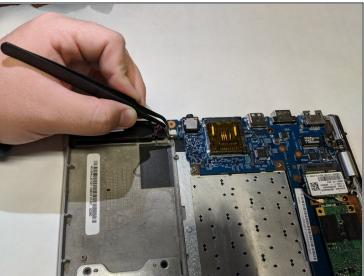
• Using a pair of <u>tweezers</u>, remove the two cables connecting both speakers to the motherboard panel.
