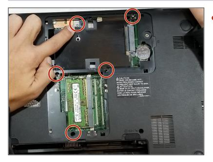
• Remove the remaining five 10mm PH#1 screws within access panel.
