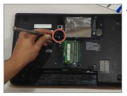
• Unscrew the 2mm PH#1 screw next to the Toshiba Device information tag.
