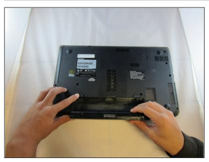
• Pull battery free from device and release switch 2.
