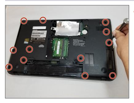
• Unscrew the twelve 5mm PH#1 screws on the bottom of the device.
