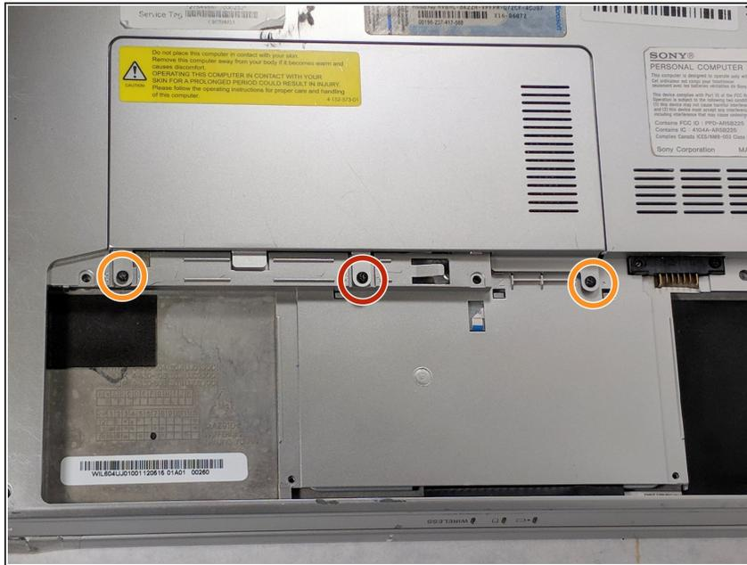
**i** The Hard Drive bay cover has three Phillips head screws at two different lengths. Be sure to organize your screws, as improper replacement will result in damage to your device.
