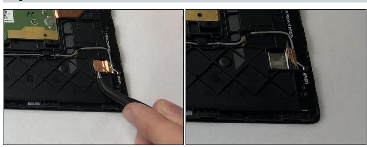
• Locate the copper foil holding down the WiFi module near where the grey wire connects. Use <u>tweezers</u> to carefully lift up and separate the copper foil.
