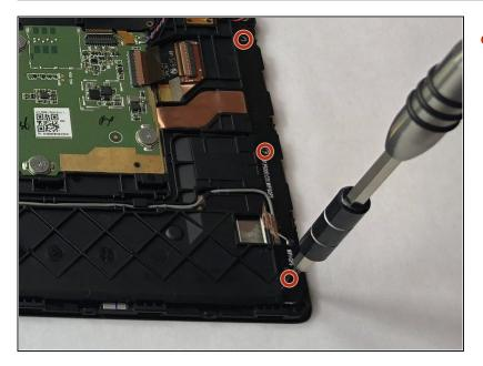
Remove the three 2mm screws holding the wifi module to the device using a PH00 screwdriver.
