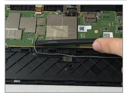
Locate the WiFi module connection on the motherboard by following the grey wire along the bottom.
