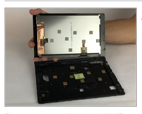
Lift the LCD out with your fingers, being careful that the wires do not catch. To reassemble your device, follow these instructions in reverse order.
