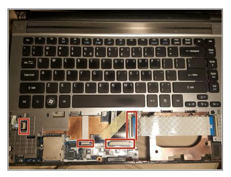
Next, disconnect the 4 wired tapes of the keyboard from the motherboard just like we did with the lower front touchpad panel.
