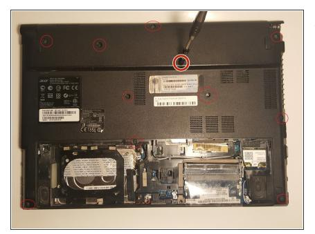
Remove the eleven screws that hold that back panel to the laptop using a J0 Phillips screwdriver bit.
