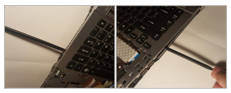
Finally, using an opening tool, gently pry along the edge of the keyboard to separate it from the laptop.
