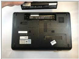
Carefully lift the battery out and away from the laptop.
