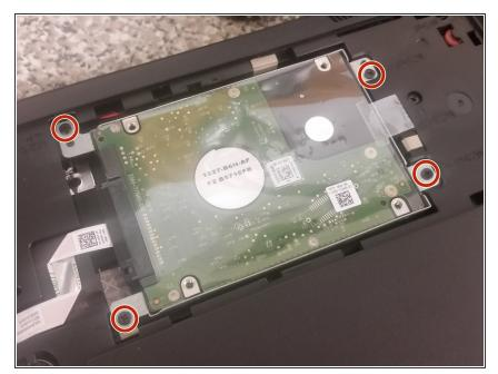
Remove the four Philips screws securing the hard drive caddy.
