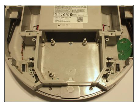
Once the fan has been removed you can take a damp cloth and clean the cavity before attaching the new device
