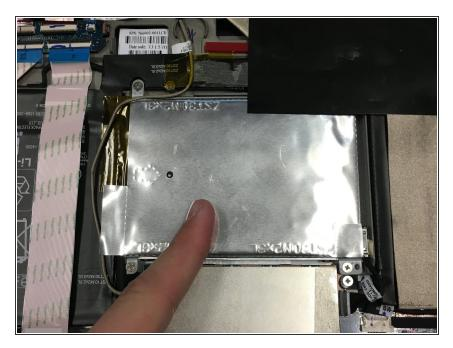
Locate the hard drive. (The hard drive is located in the center of the device)
