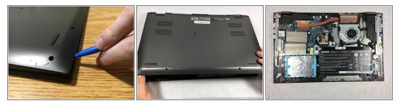
$\bigwedge$  Be careful to not crack the panel where the USB and power cord ports are.
